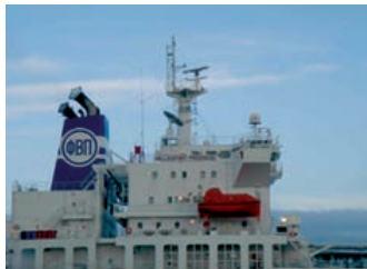
The Hellespont Progress (right) has installed the C-Bird antenna, designed to be used without a radome (centre of picture, left)
